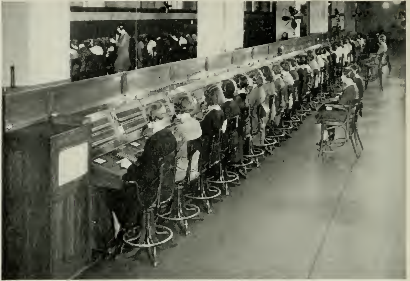
OPERATORS IN DIAL CENTRAL OFFICES HELP IN HANDLING CALLS BETWEEN MANUAL AND DIAL TELEPHONES AND TO POINTS OUT OF TOWN
